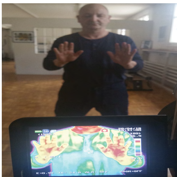
Figure 1: Measuring principle applying an infrared camera to monitor probands temperature distribution of the body part under test: in this case the hands of the seiki therapist Mr. Damljanovic.
