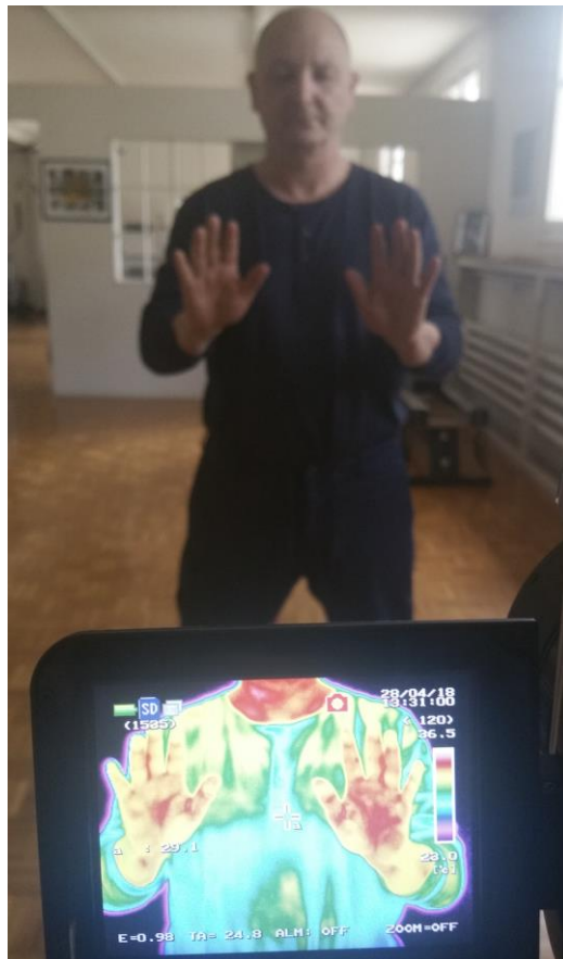
Fig.1 Measuring principle applying an infrared camera to monitor probands temperature distribution of the body part under test: in this case the hands of the seiki therapist Mr. Damljanovic.
